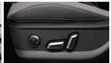
Driver's Seat with 8-direction Electric Adjustable
